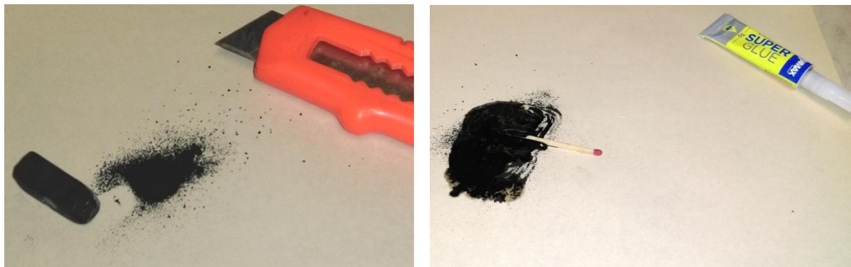
L-R: Graphite (artist's charcoal) and dust. Paste of CA glue and graphite dust
