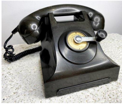
British 400 series magneto telephones - note similarity to 334
