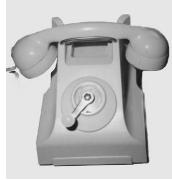
British 400 series magneto telephones - note similarity to 334
