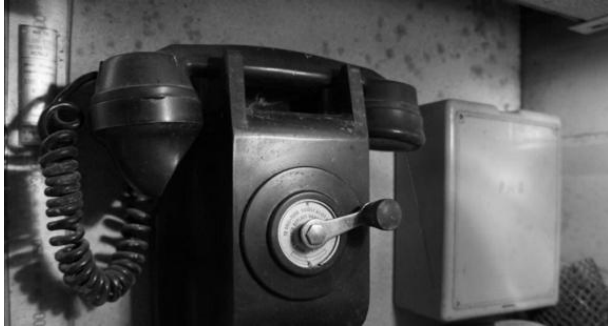
L: Battery box to right of wall phone. R: Cover off showing 2 x no 6 cells
