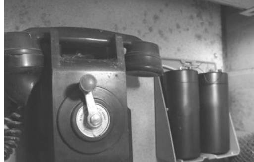
L: Battery box to right of wall phone. R: Cover off showing 2 x no 6 cells
